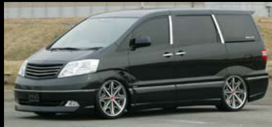
■ ALPHARD LOW DISK 21inch F 8.5J+49 R 9.5J+36 TIRE F 245/35-21 R 285/30-21 LOW DOWN
