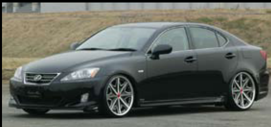
■ LEXUS IS 250 LOW DISK 20inch F 8.0J+32 R 9.0J+32 TIRE F 225/30-20 R 235/30-20 LOW DOWN
